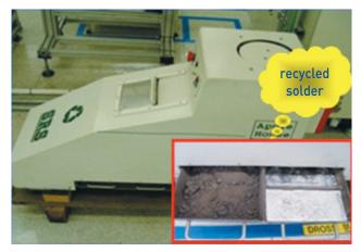
The recycling equipment of waste solder
