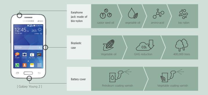
The first secret is the earphone jack. The part wrapping the earphone jack of 'Galaxy Young 2' uses eco-friendly materials. It is a plastic-like material that is a mixture of 20% bio-nylon, made by adding castor seed oil for stronger heat resistance, and hygroscocipity and petroleum resin. This process saves production cost by 10% compared to when using the original heat-resistant polyamide (PA9T) material.
