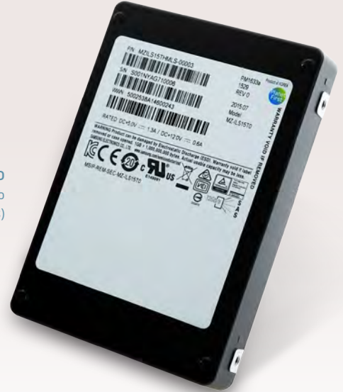
15.36TB SAS SSD (equipped with 512 of 256Gb V-NAND memory chips)
