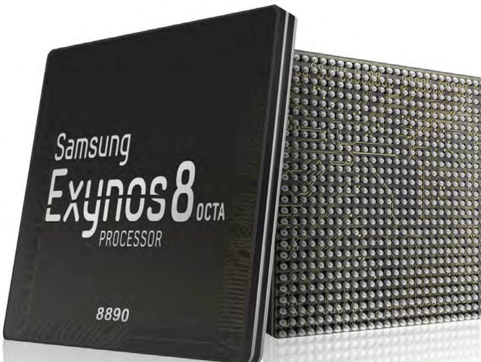
Exynos 8 Octa (8890), 2nd generation 14nm-based, integrated one-chip solution for mobile devices
