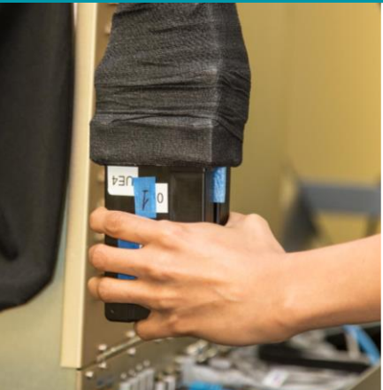
Handheld and in-vehicle UEs with hand-blocking
