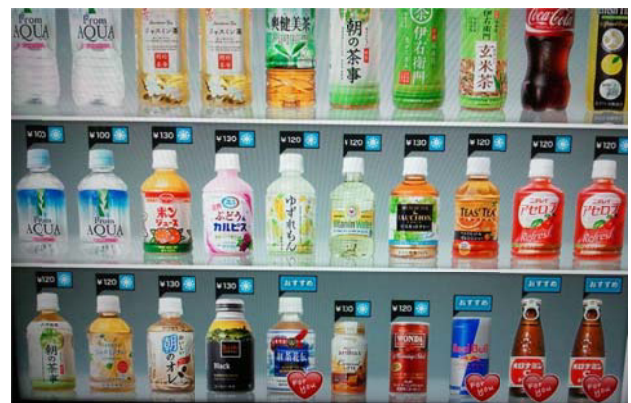
Figure 10. Screen of a vending machine with recommendations about beverages (the red heart icon indicates recommended drinks) based on customer photos transmitted over a WiMAX connection. (Source: Senza Fili)
