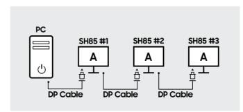
Daisy chain function allows extension and replication in multi-monitor settings with just a single DP cable connection.
