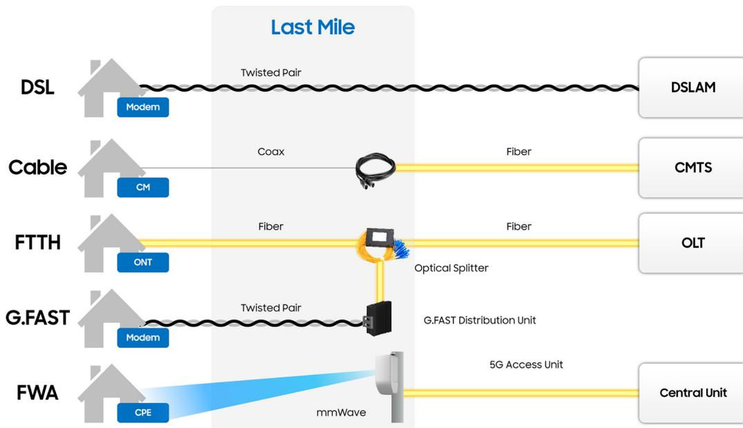
Figure 1: Wireline technologies compared to mmWave FWA
