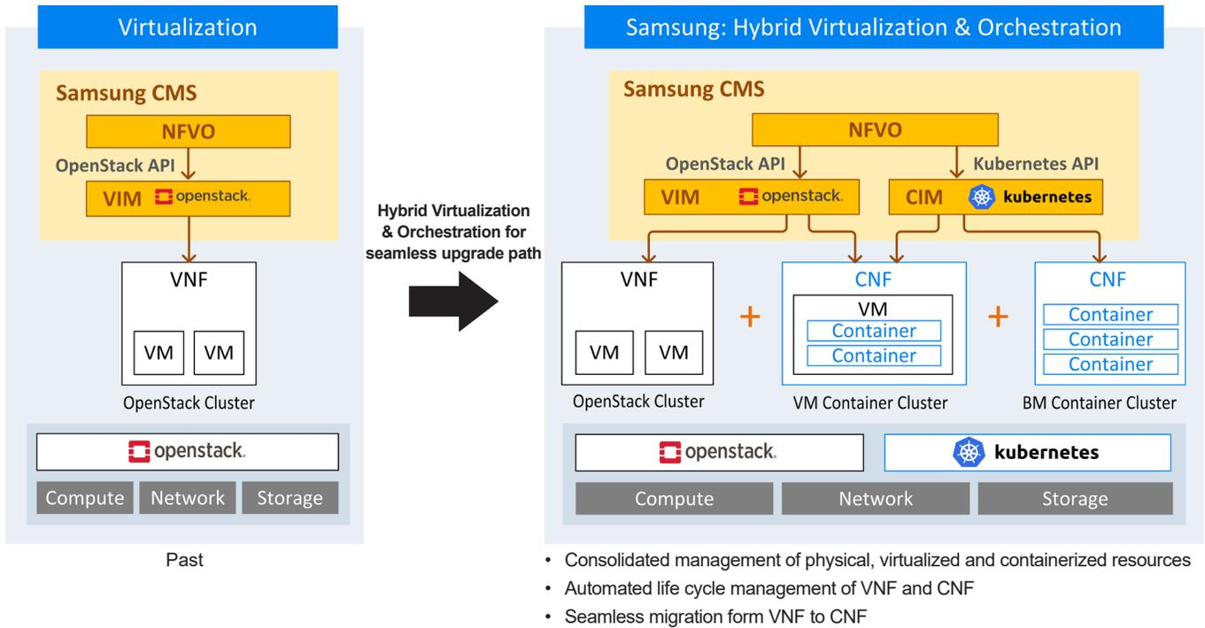
Figure 4-4. Hybrid Virtualization and Hybrid Cloud Orchestration
