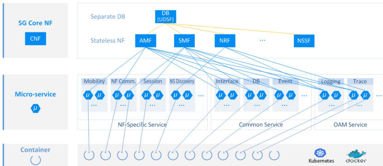
Figure 4-3. Samsung 5G Core : Cloud Native Architecture
